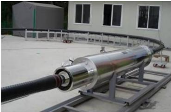
HTS Cable Joint
